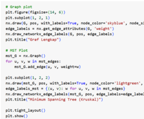
Figure 5. The Part of Source Code for Determine the MST (Kruskal Algorithm)
